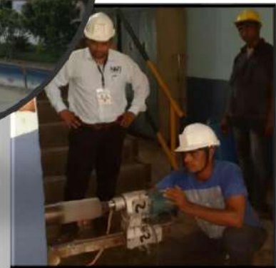
CORE CUTTING TEST
